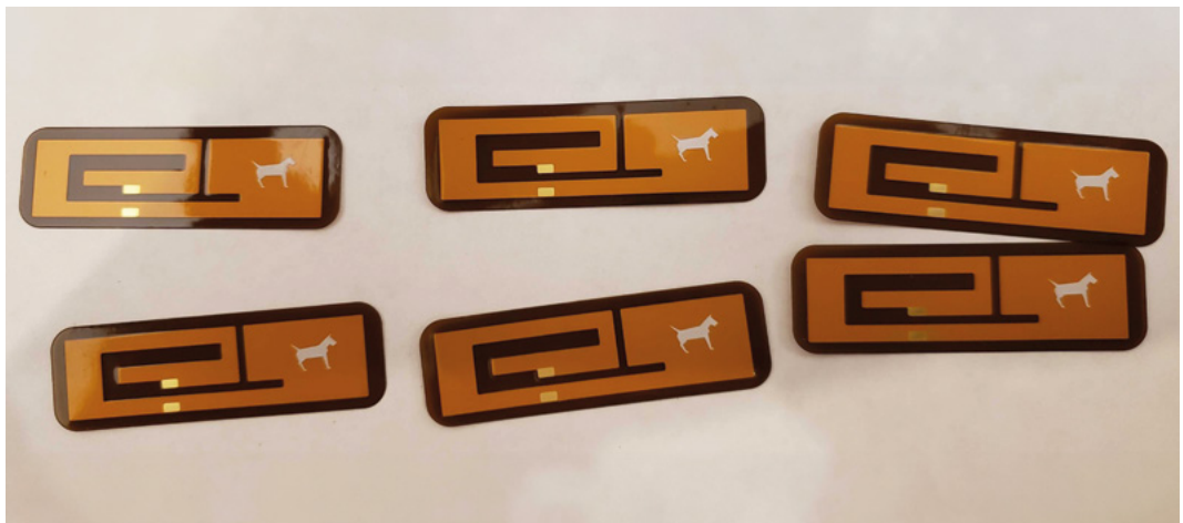
Right ♦ Some small polyamide flexible PCB antennas fabricated by OSH Park
